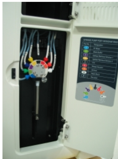
Figur 2-6: Spruta bakom luckan
