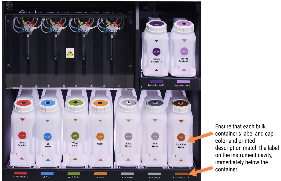
Figure 2-15: BOND-III bulk reagent containers in position
