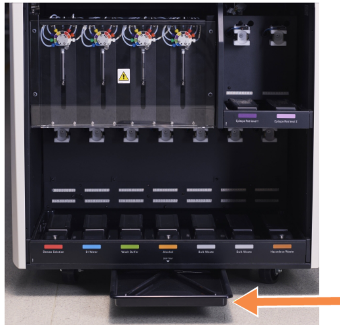
Figure 12-14: The BOND-III Processing Module drip tray
