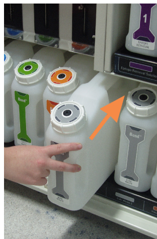
Figure 12-1: Returning the waste container to its position
