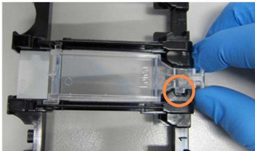
Figure 4-6: Positioning a Covertile on a slide
