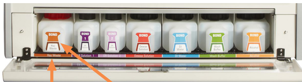
Figure 2-17: BOND-MAX bulk reagents in position
