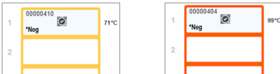
Figure 5-6: Temperature-indication borders of the slide trays: warm (left) and hot (right)
