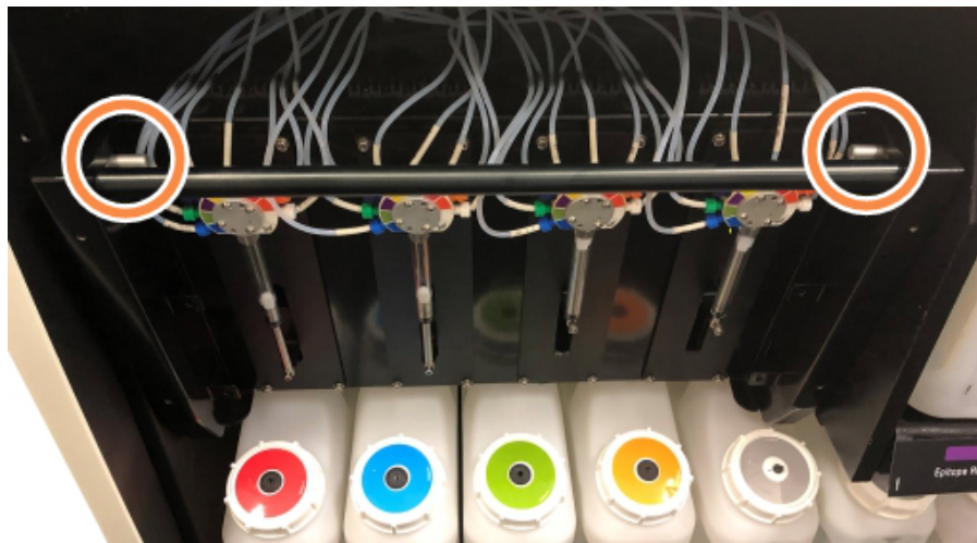
Figure 12-9: Location of release pins with unit open for access
