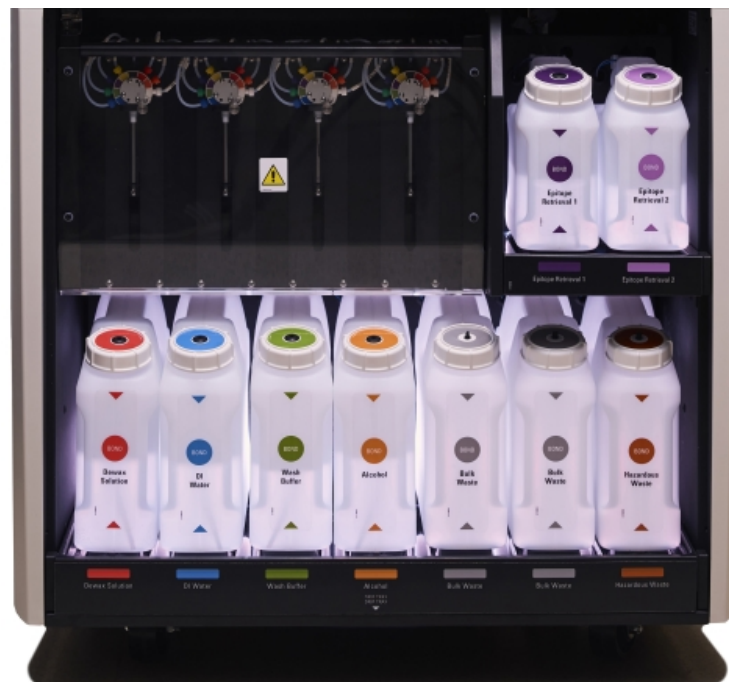
Figure 2-16: Bulk container lighting system
