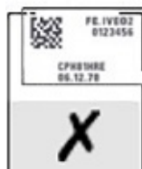
Figure 6-6: Place the label within the edges of the slide
