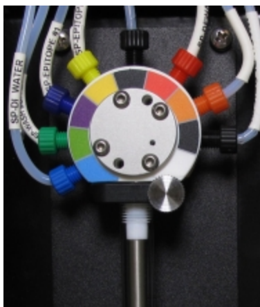
Figure 2-24: BOND-MAX 9-port syringe
