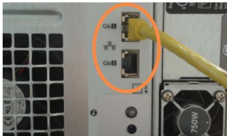
Figure 16-5: Ethernet ports used for LIS connectivity
