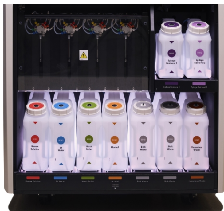
Figure 2-16: Bulk container lighting system
