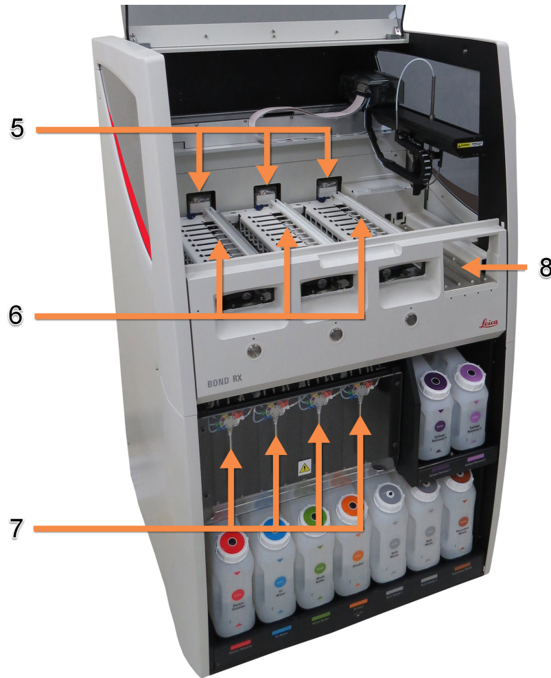
Figure 2-2: The front of the BOND RX Processing Module
