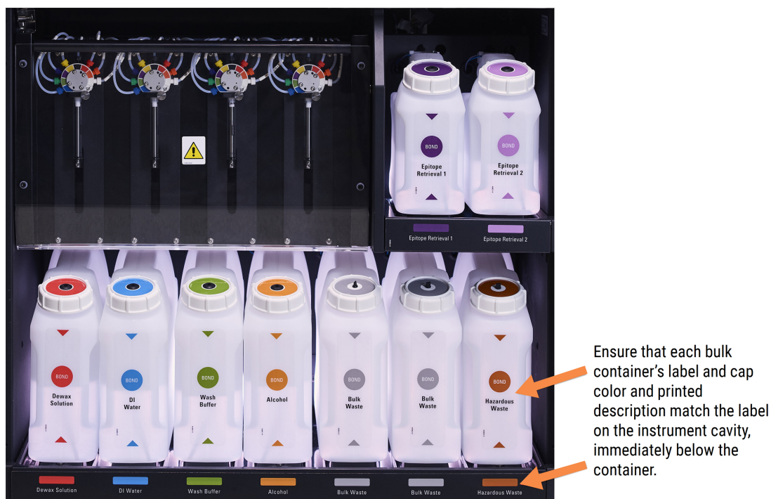
Figure 2-15: BOND RX bulk reagent containers in position
