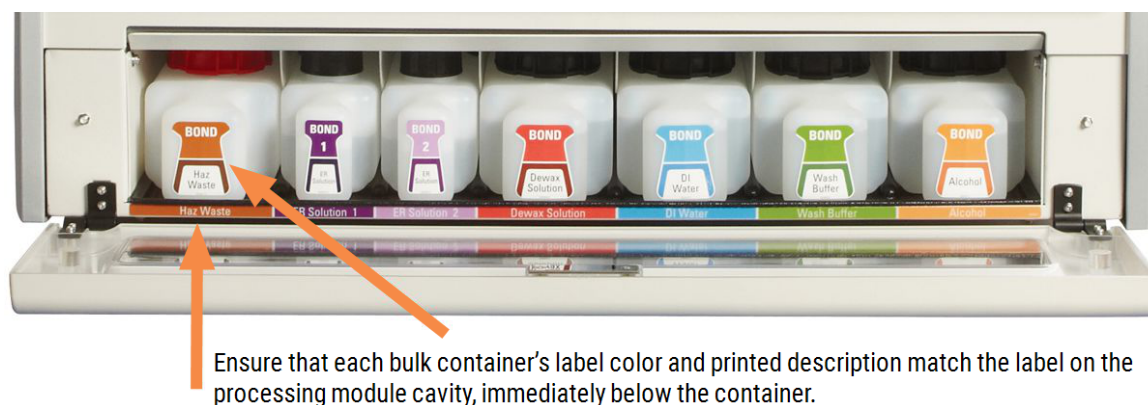
Figure 2-17: BOND RX m bulk reagents in position
