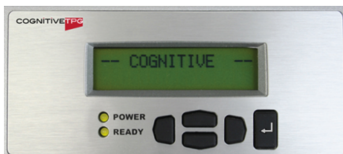
Figure 17-1: Cognitive Printer LCD display and keypad
