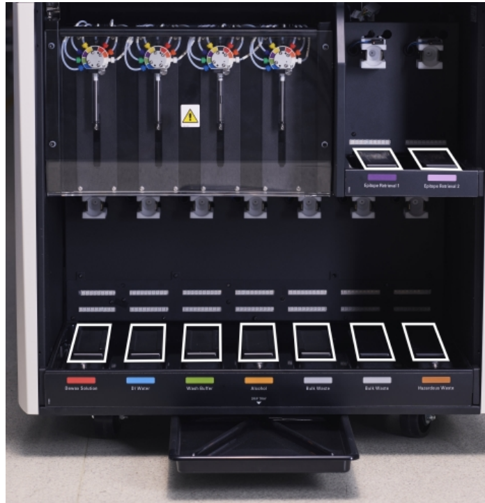
Figure 12-13: BOND RX bulk container drip trays showing the weight sensor covers
