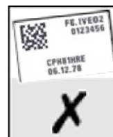
Figure 6-6: Place the label within the edges of the slide
