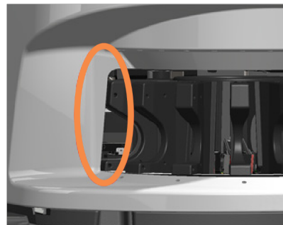
Figure 6-8: Pinch points on either edge of rack loading area
