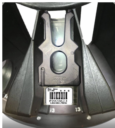
Figure 6-20: Rack inserted fully into the carousel
