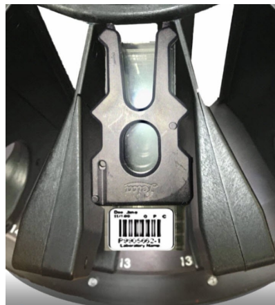
Figure 6-10: Rack inserted fully into the rack slot
