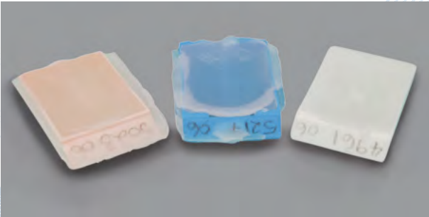
Blocks that have resulted from over-filling the molds during embedding.
